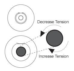
Ribbon wrinkling may also be alleviated by adjusting the eccentric at the end of the ribbon guide shaft located at the lower, rear section of the print station. Loosen the screw securing the shaft and using a wrench, turn the eccentric until wrinkles have been eliminated then retighten the screw to secure the shaft.
